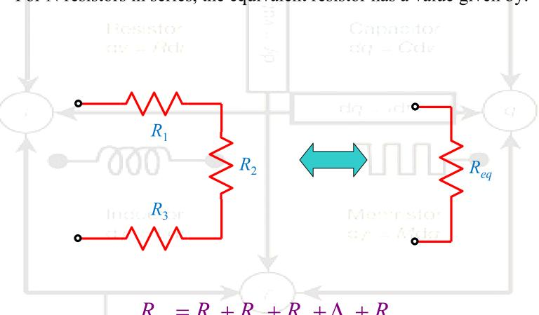
$$R_{eq} = R_1 + R_2 + R_3 + \Lambda + R_N$$
