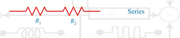
➤ If we wish to replace the two series resistors with a single <u>equivalent</u> resistor whose voltage-current relationship is the same, the *equivalent* resistor has a value given by
